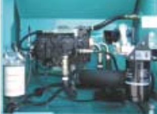
Firewall separates the pump compartment from the engine
